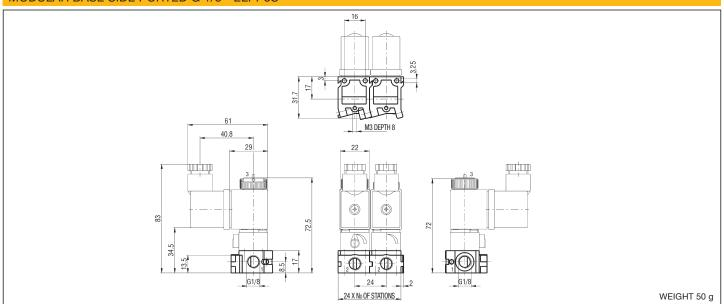
HOW TO ORDER A SOLENOID VALVE COMPLETE OF COIL AND BASE Example: 3/2 N.C. solenoid valve base mounted (with manual override) + coil 24 V D.C. - ELPP8S/P/USB/02400
